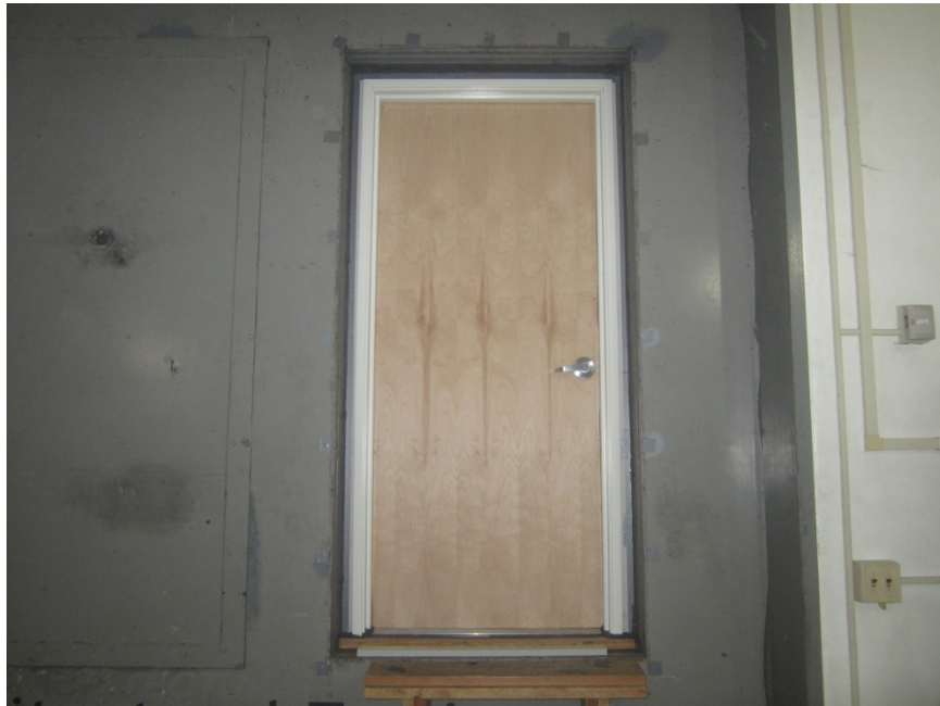
Source Room View of an Installed Test Specimen
